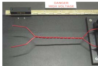
Twisted Pair specimen used in Dielectric Breakdown Test
